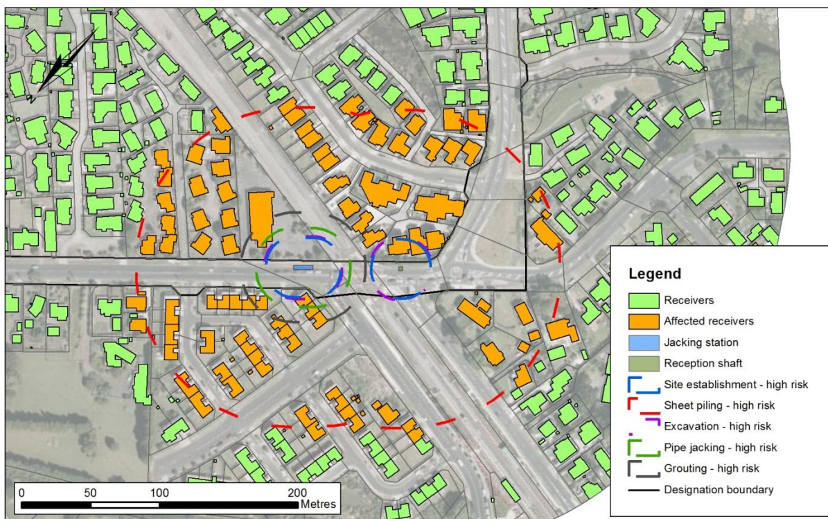
Figure 6 Extent of affected properties at the North Auckland railway crossing due to trenchless construction activities
